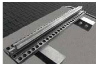
Type A: Spin holes in one line
